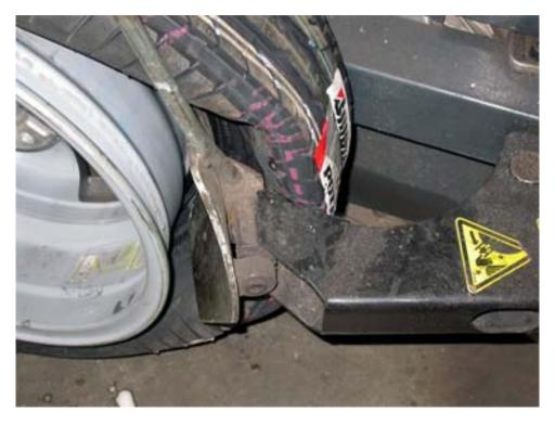
Consequence: discard tyre for risk of long-term damage caused by separation in tyre structure
