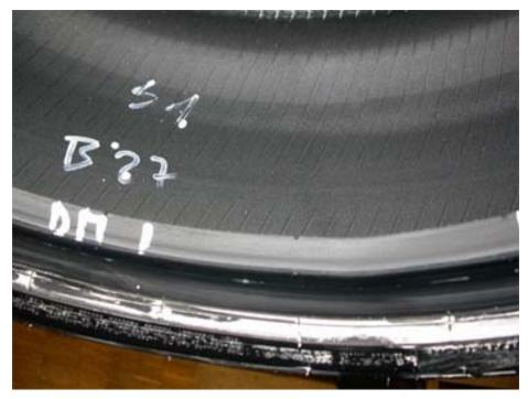
Consequence: check inner liner for damage and bead for broken core
