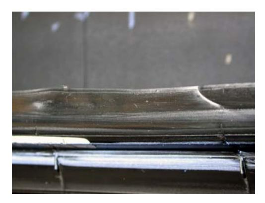
Consequence: check inner liner for damage (also see inner liner damages); check tyre for leaks
