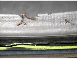
Consequence: if minor scratches are found in the rubber, tyre can be used again; if scratches reach as far as to the ply: discard tyre
