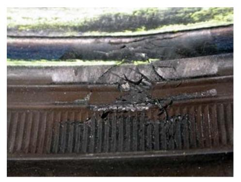
Consequence: check tyre for leaks; when damaged as far as to the ply, discard tyre
